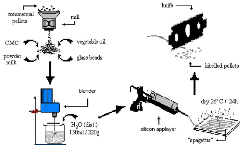
**Figure 1.** Schematic representation of the labelled pellets preparation.
